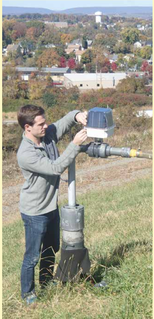
Greg fine tuning one of his patent-pending landfill gas well monitoring devices.
