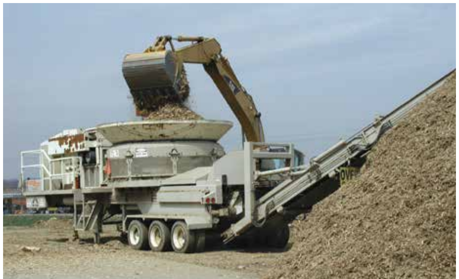
The landfill's industrial-strength grinder turns collected hardwood waste into double-ground mulch.
